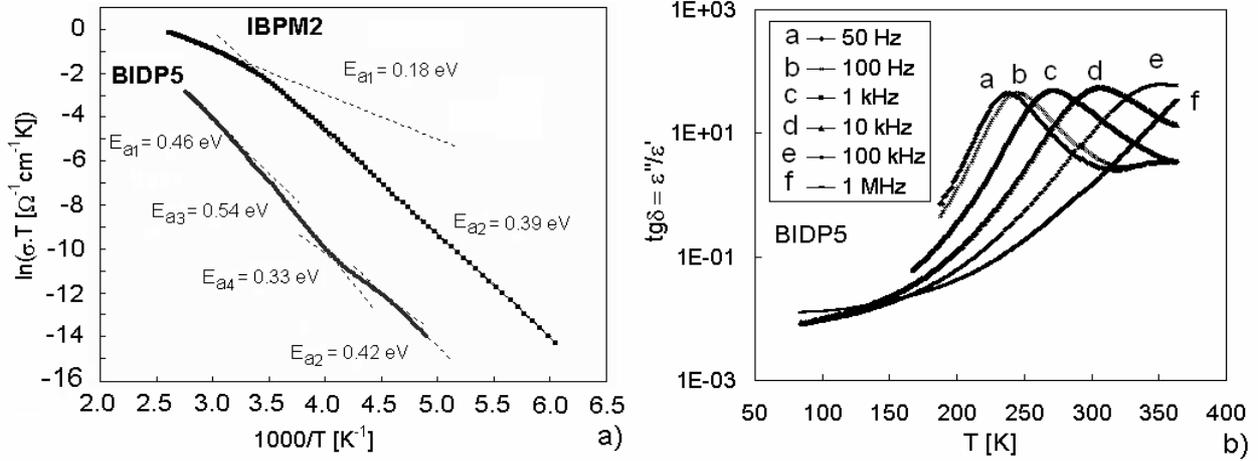
Fig. 1. Representative dc electrical results obtained on BIDP5 ( $x = 9.09$ ) and IBPM2 ( $y = 3.125$ ) samples including Arrhenius plot of dc conductivity and temperature dependence of dielectric loss tangent (b) for sample BIDP5.
