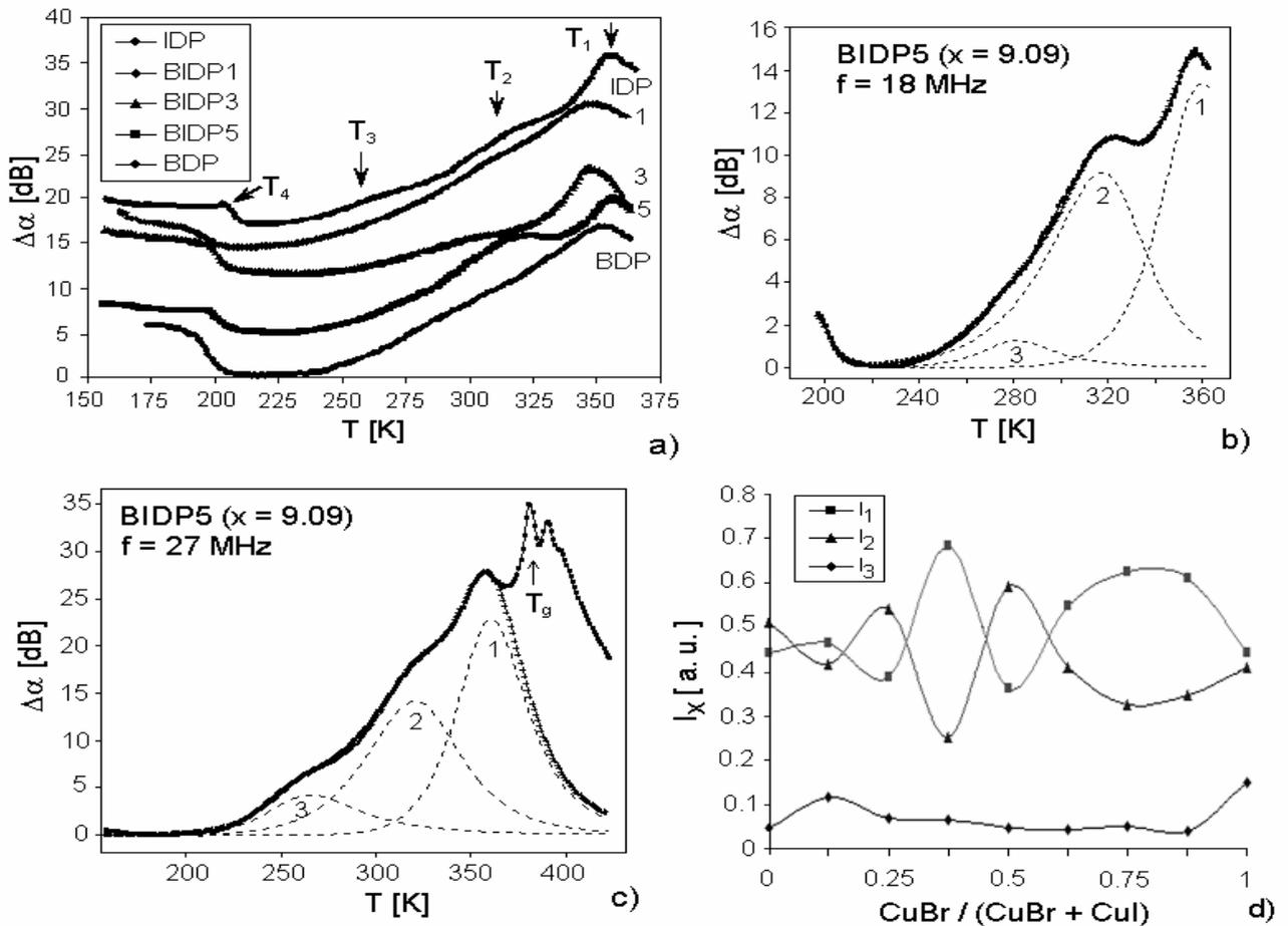
Fig. 2. Acoustics attenuation spectra of several glasses of the System I (a), representative acoustic spectra of sample BIDP5 measured at 18 MHz (b) and 27 MHz (c) and the dependence of the relative peak intensities on glass composition (d). Cross-marked lines represent the best fit as superposition of individual peaks (dashed lines).
